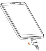
It is advised that you fully charge your battery before first use ( 1000 ). Connect the charger to your phone and an outlet. Charging status is indicated by the percentage on screen while the phone is powered off. The percentage increases as the phone is charged.
